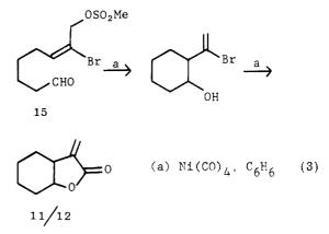
the zero valent reagent serves two different roles. Treatment of allylic methanesulfonate ester 15a with excess nickel carbonyl under conditions favoring complete conversion (95 h, 65 °C, benzene) gave a mixture of 11 and 12 (2:1 ratio) in 58% yield. At shorter reaction times, the intermediate vinyl bromide alcohols (3 and 4) can be isolated. Treatment of 15b with nickel carbonyl for 28 h at 65 °C in benzene afforded 3 and 4 (2:1, 49% isolated vield) and minor amounts of 11 and 12 (2:1, 9%).
